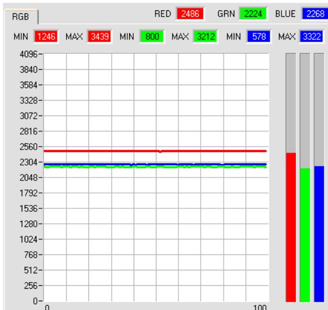
When the red channel becomes higher than 2000, output OUT0 switches to HI. When it is lower than 2000, the output switches to LO.
